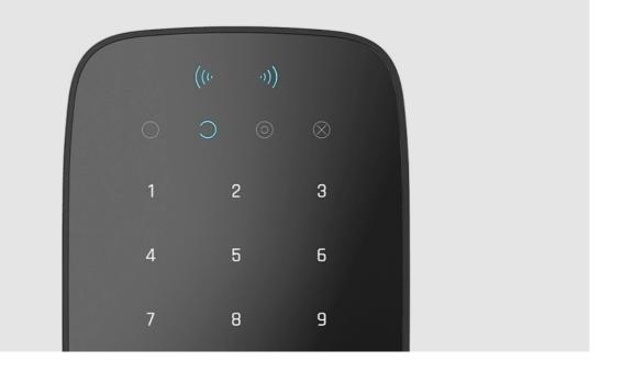
You can use the KeyPad Plus without ambient lighting as the keypad has a backlight. The pressing of the buttons is accompanied by a sound signal. The backlight brightness and keypad volume are adjustable in the settings. If you do not touch the keypad for 4 seconds, KeyPad Plus reduces the backlight brightness, and 8 seconds later goes into power-saving mode and turns off the display.
